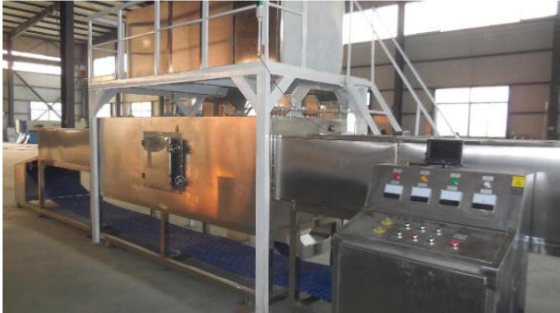
Configuration of LD1706 microwave frozen block thawing equipment:
